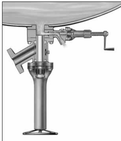
Fig. 2 - Drain Valve Open for Sample
