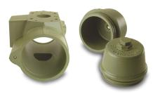
The XL Commando range solves aggressive corrosion problems. It works where stainless doesn't. A proprietary heat treatment with CG941 fluorpolymer impregnates the body making it impervious to corrosion. The steel pinion is also fluorpolymer coated. Field service has shown that the Commando actuators outperform other actuators in corrosive environments.
